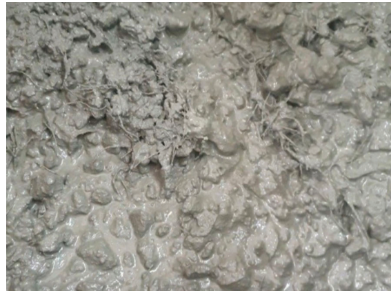
Fiber Reinforced Concrete
